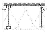
FINISHED FLOOR - VARIES SHEATHING PER STRUCTURAL 11 7/8" TJI JOISTS PER STRUCTURAL R-38 BATT INSULATION AT GARAGE ACOUSTICAL INSULATION AT BATHROOMS AND BEDROOMS GYPSUM CEILING BOARD 5/8" TYPE-X AT GARAGE CEILING/BEAMS INTERIOR FINISH
