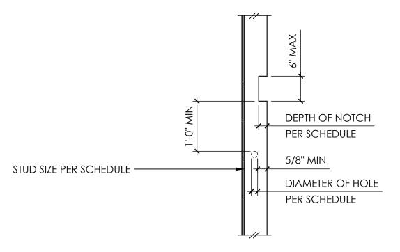
TYPICAL ALLOWABLE HOLES AND NOTCHES IN WALL STUDS
