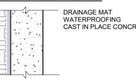
CAST IN PLACE CONCRETE WALL
